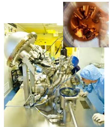
Small-Spot Röntgen-Photoelektronen-Spektrometer und Analysenkammer (rechts oben) im Reinraum Small-Spot Parallel Angle Resolved X-Ray Photoelectron Spectrometer (XPS) and Analytic Chamber (right) in Clean Room Environment
