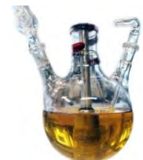
Sensorsystem (im Ölbad) zur Ölzustandsüberwachung / Sensor System (in oil bath) for Oil-Condition-Monitoring
