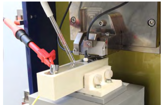
Tribokorrosionsaufbau im Kleinlast-Tribometer Electrochemical-Cell-Unit at the Low-Load Tribometer
