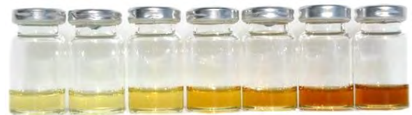
Öl in verschiedenen Alterungsphasen (von links nach rechts) / Oil in different conditions during artificial alteration (from right to left: increasing degree of deterioration)
